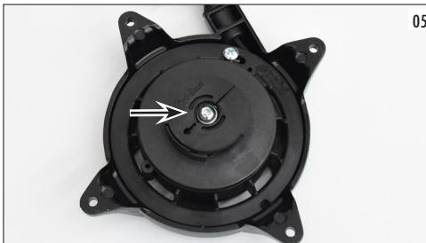
**⚠ CAUTION!** Under the cover there are two teeth for the starter jaw (check their condition and if worn replace them), under them 2 small calipers. Be very careful not to lose these small parts.
