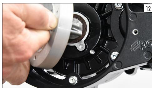
Screw the flywheel nut without locking it so that the crankshaft can rotate in the flywheel. Screw the dial gauge support into the spark plug hose, insert the dial gauge and move the piston to the top dead centre. Now reset the dial gauge and rotate the crankshaft anti-clock wise of 3,7 mm towards the flywheel sense (see arrow in photo 13).
