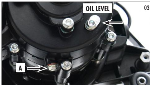
Check that the oil level reaches the lower edge of the level hole. If there is too much oil, let it flow out from the hole until it stops flowing and collect the oil in a suitable container. If there is not enough oil, top up as required through the breather hole located at the top. After checking it, tighten the screws. Use ELF Moto Gear Oil 10 W 40 ANTI Clutch Slippage or Shell advance gear SAE 10 W 40 API GL-3
