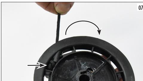
Now insert the plastic wheel in its housing again, and check through the hole that the internal spring hook is perfectly coupled (Photo 8), place the springs, the teeth for the starter jaw and screw the cover again using medium thread-locker.
