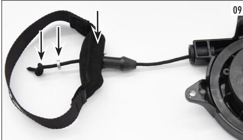
**ATTENTION:** verify that the return spring does not reach the end of the stroke. Pull the rope completely and turn the wheel again to check that it can make at least one turn before stopping.
