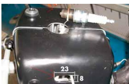
must be replaced by the thermocouple sensor washer. Now place the spark plug again and screw it being careful not to damage the small cable welded to the washer itself. Now close the hole for the thermocouple cable passage using the small rubber supplied, as shown in the picture.
