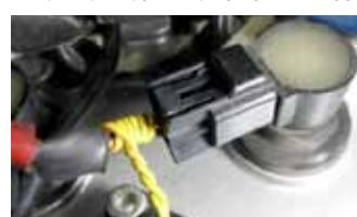
Connect the yellow RPM cable as shown . Wind up from 0 to 10 turns (spire); more turns more sensitive.
